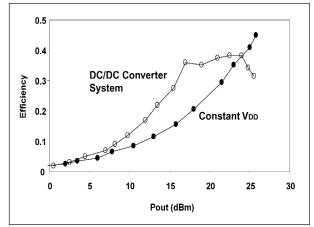
Figure 32 · Efficiency of a GaAs FET envelopetracking transmitter.
