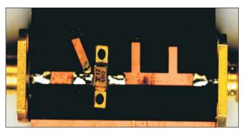
Figure 14 · Example X-band class-E PA.
