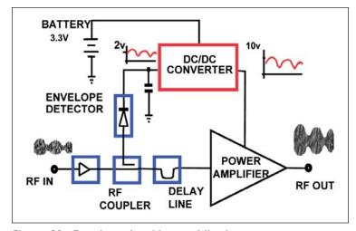
Figure 31 · Envelope-tracking architecture.
