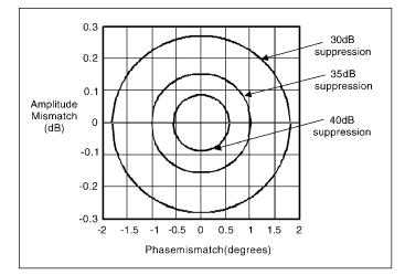
Figure 47 · Gain/phase matching requirements.
