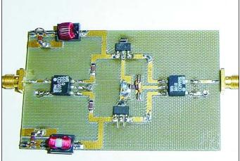
Figure 61 · Prototype class-D PA for delta-sigma modulation (courtesy UCSD).
