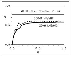
Figure 27 · Efficiency of Kahn-tecnique transmitters.
