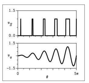
Figure 59 · RF pulse-width modulation.
