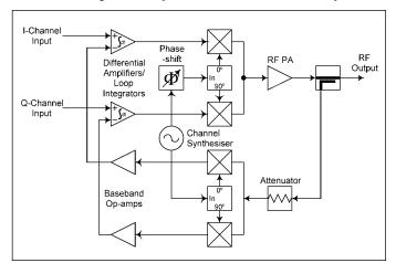
Figure 44 · Cartesian-loop transmitter configuration.
