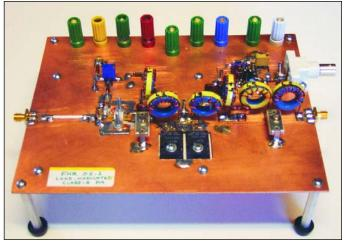
Figure 70 · Load-modulated class-E PA (courtesy GMRR).
