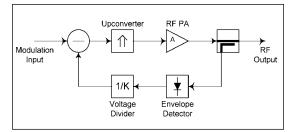
Fig 41 · Envelope feedback applied to a complete transmitter.
