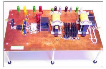
Figure 68 · Electronically tunable class-D PA (courtesy GMRR).
