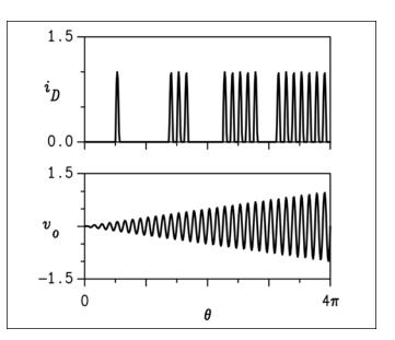
Figure 65 · Carrier pulse-width modulation.
