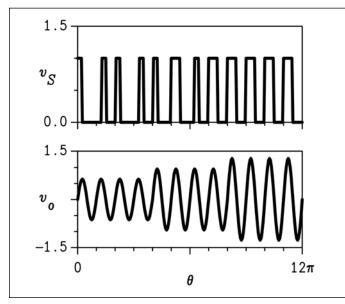
Figure 62 · Delta-sigma modulation.
