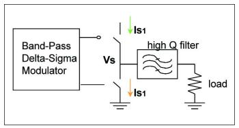
Figure 63 · Delta-sigma modulator.
