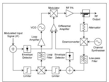
Figure 43 · Block diagram of a polar-loop transmitter.
