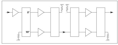
Figure 21 · Amplifier stages with quadrature combiners.
