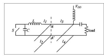
Figure 13 · Idealized microwave class-E PA circuit.
