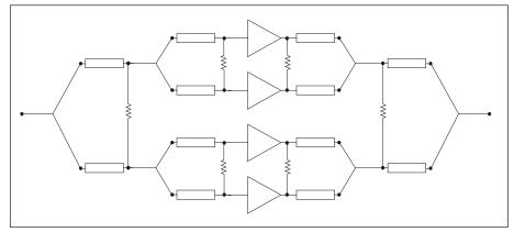
Figure 22 · Multi-section Wilkinson combining architecture.
