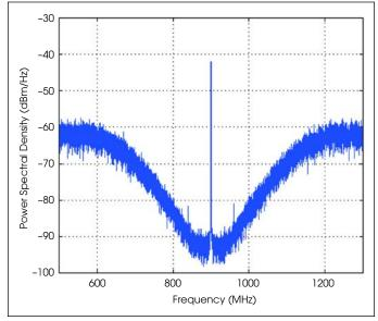
Figure 64 · Spectrum of delta-sigma modulation.
