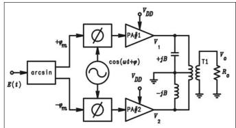
Figure 36 · Chireix-outphasing transmitter.
