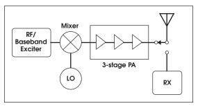
Figure 20 · A conventional transmitter.
