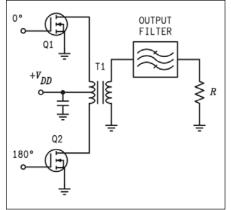
Figure 8 · Transformer-coupled push-pull PA.
