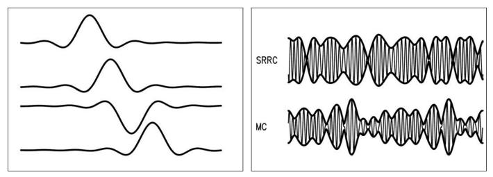
Figure 1 · SRRC data pulses.
