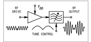
Figure 69 · Load modulation by electronic tuning.
