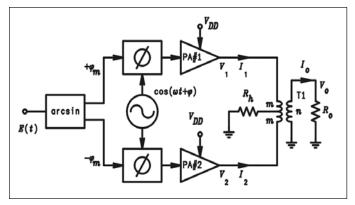
Figure 33 · Hybrid-combined outphasing transmitter.
