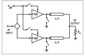
Figure 66 · Switched PAs with quarter-wavelength transmission line combiner.
