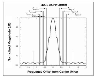
Figure 3 · ACPR offsets and bandwidths.
