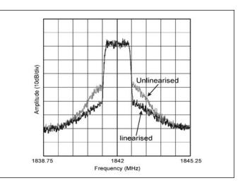
Figure 52 · Linearization by diode-based RF predistorter (courtesy WSI).
