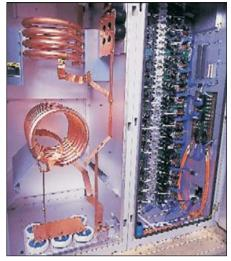
Figure 15  $\cdot$  3-kW high efficiency PA for 13.56 ISM-band operation. (Courtesy Advanced Energy)
