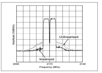
Figure 57 · Linearization of 3G W-CDMA PA signal by digitial baseband input predistorter (courtesy WSI).
