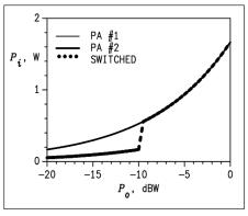
Figure 23 · Power consumption by PAs of different sizes.
