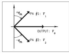
Figure 34 · Signal vectors in outphasing.
