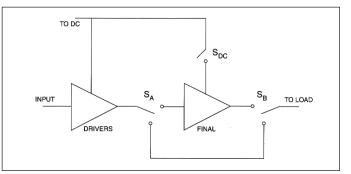
Figure 24 · Stage-bypassing architecture.
