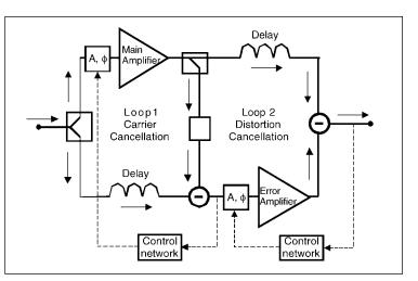
Figure 46 · Block diagram of a feed-forward transmitter in its basic form.
