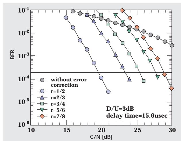
Figure 14: Multipath characteristics (C/N vs. BER)
