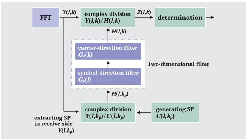
Figure 9: Demodulation process using SPs
