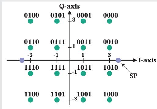
Figure 8: Sp data of 16QAM-OFDM (for the RMS value  $\sqrt{10}$  in 16QAM, SP is placed at  $(+L \sqrt{10}, 0)$  or  $(-L \sqrt{10}, 0)$ )
