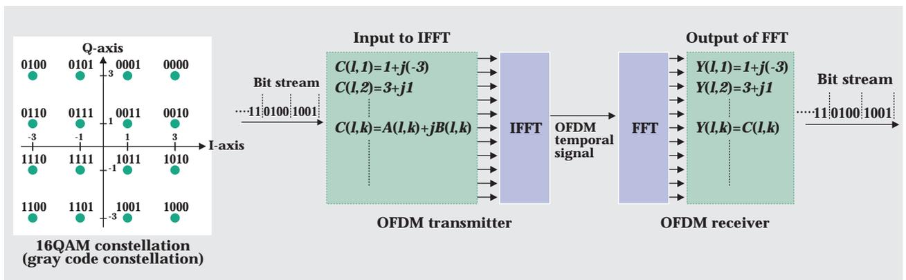
Figure 4: OFDM transmit signal (case of 16QAM-OFDM)
