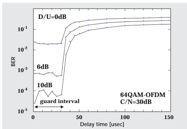
Figure 13: Multipath characteristics (delay time vs. BER)
