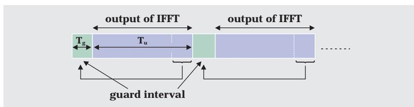
Figure 2: Attaching a guard interval
