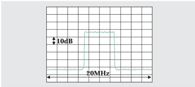
Figure 3: OFDM transmission spectrum
