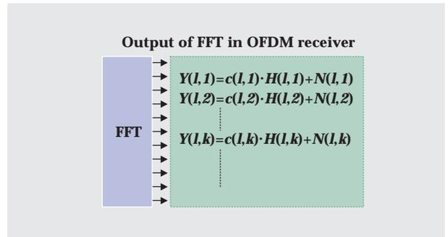
Figure 6: Output of FFT in OFDM receiver (frequency response  $H(l,k)$  in transmission path with noise  $N(l,k)$ )
