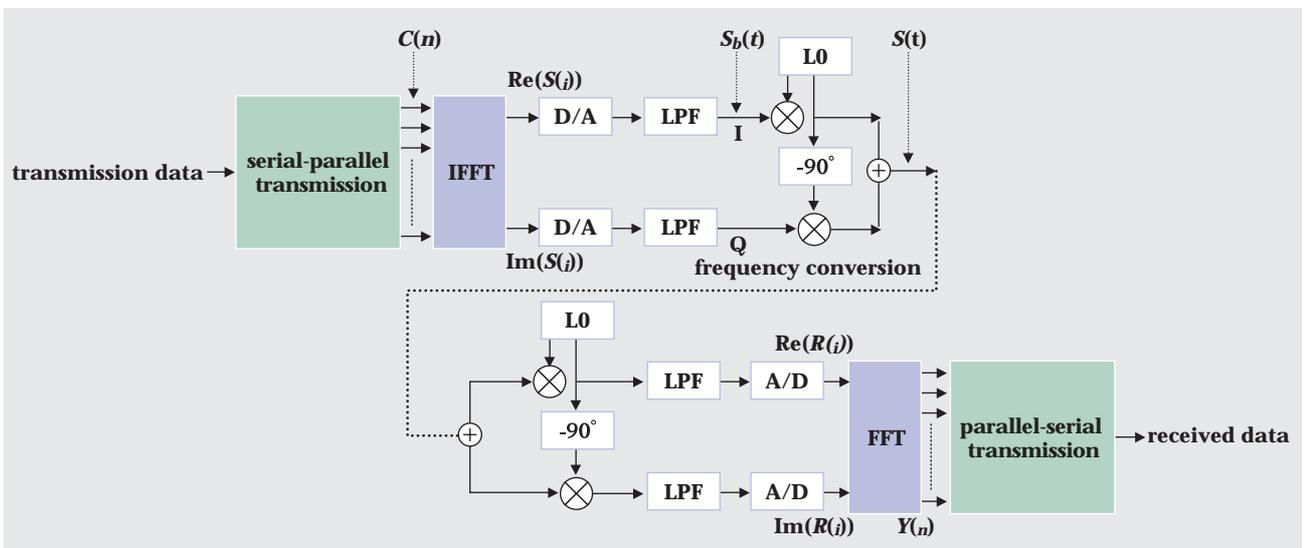
Figure 5: OFDM transmit/receive system
