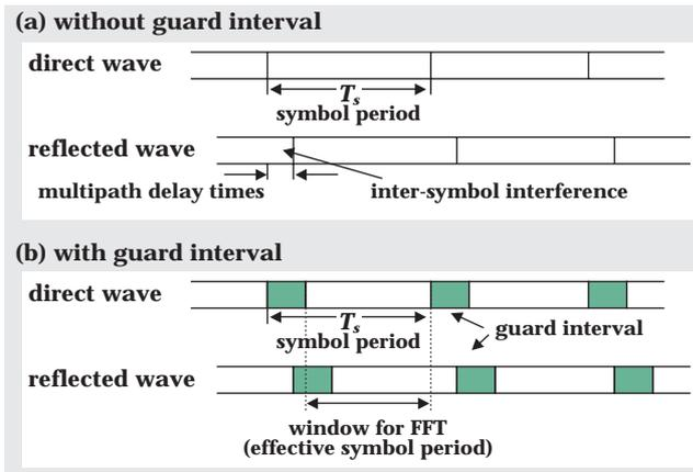
Figure 11: Guard intervals and multipath distortion
