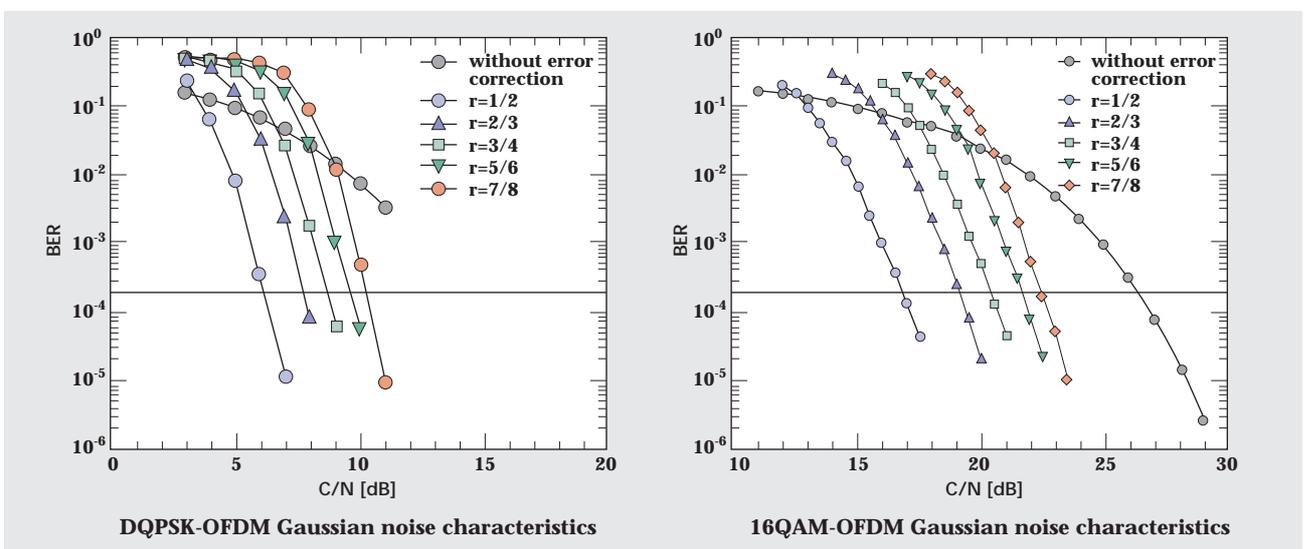
Figure 12: OFDM Gaussian noise characteristics
