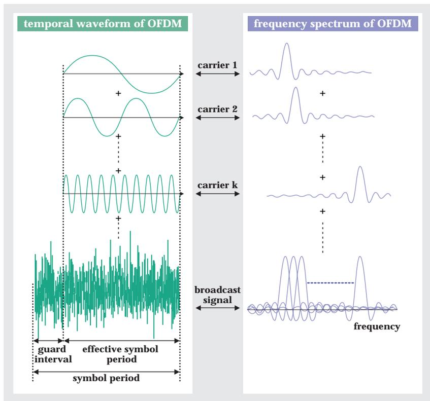
Figure 1: OFDM time spectrum and frequency spectrum
